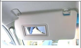
1. Remove the sun visors, grab handles and rear coat hanger hooks. Unclip the centre front interior light fitting (not shown).
