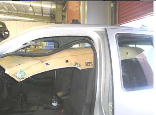
7. Carefully lower the headlining as shown in the adjacent diagram. It does not need to be totally removed.
