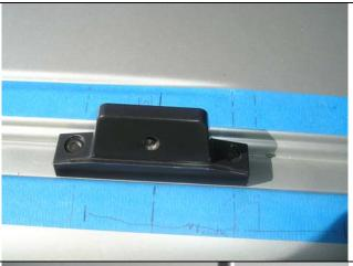
Use the rack mounting bocks supplied in the kit to mark the centre points of the holes to be drilled for the front and rear cargo barrier mounts.
