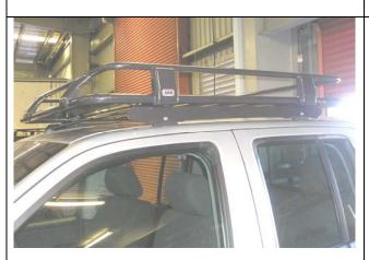
19. With the assistance of another person, lift the roof rack onto the vehicle and position evenly.
