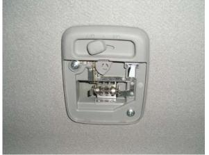
3. Remove the rear interior light housing from the ceiling.
