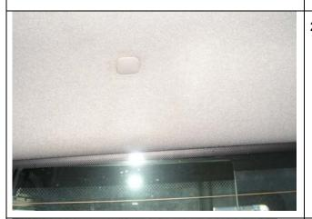
2. Remove the plugs located at the rear of the roof liner.
